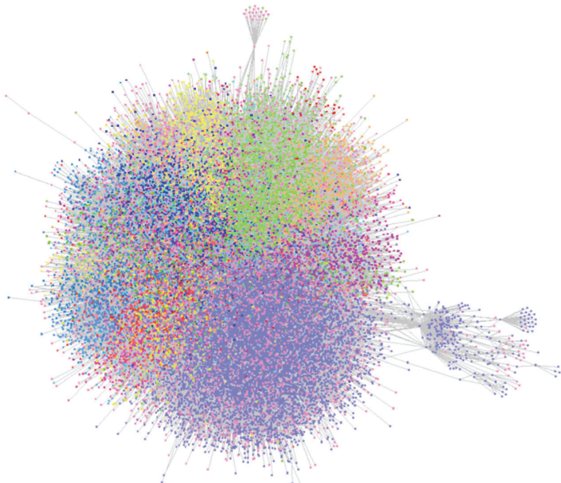
Figure 6: Internet represents a prototype of "Network of homogeneous Networks": each point represents an autonomous IP networks which color depends on the nationality of the owner. The picture has been obtained within the European Project "MOTIA" coordinated by ENEA
