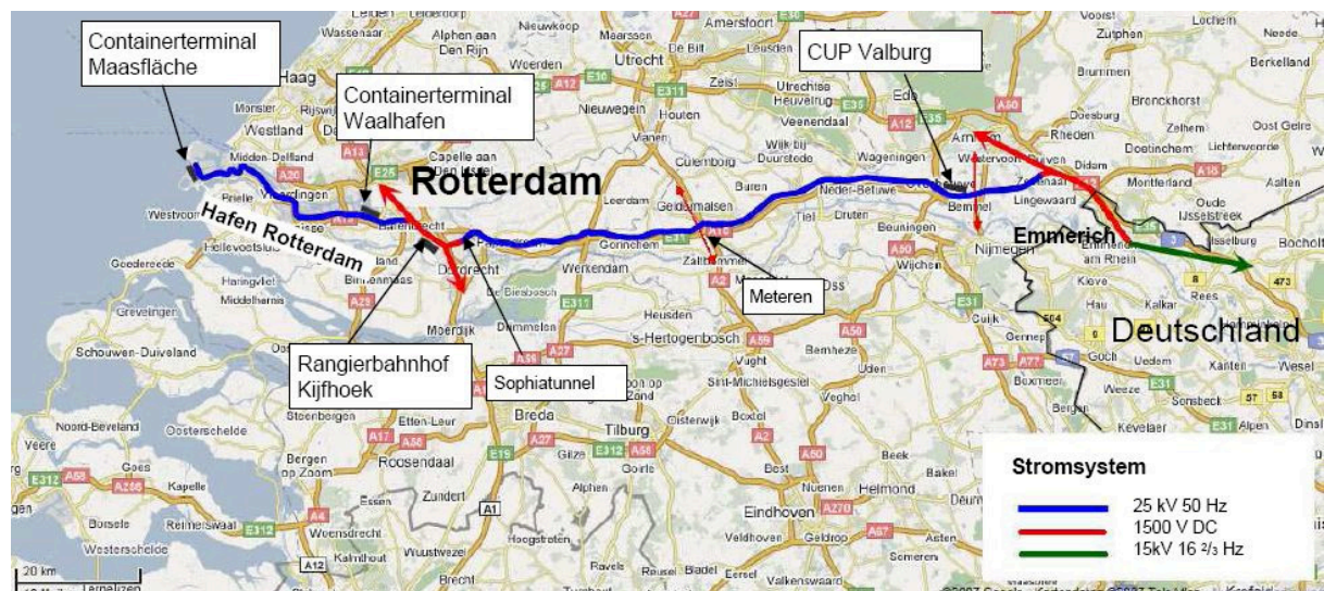
Figure 27: Electrical power systems along the Betuwe-route 23
