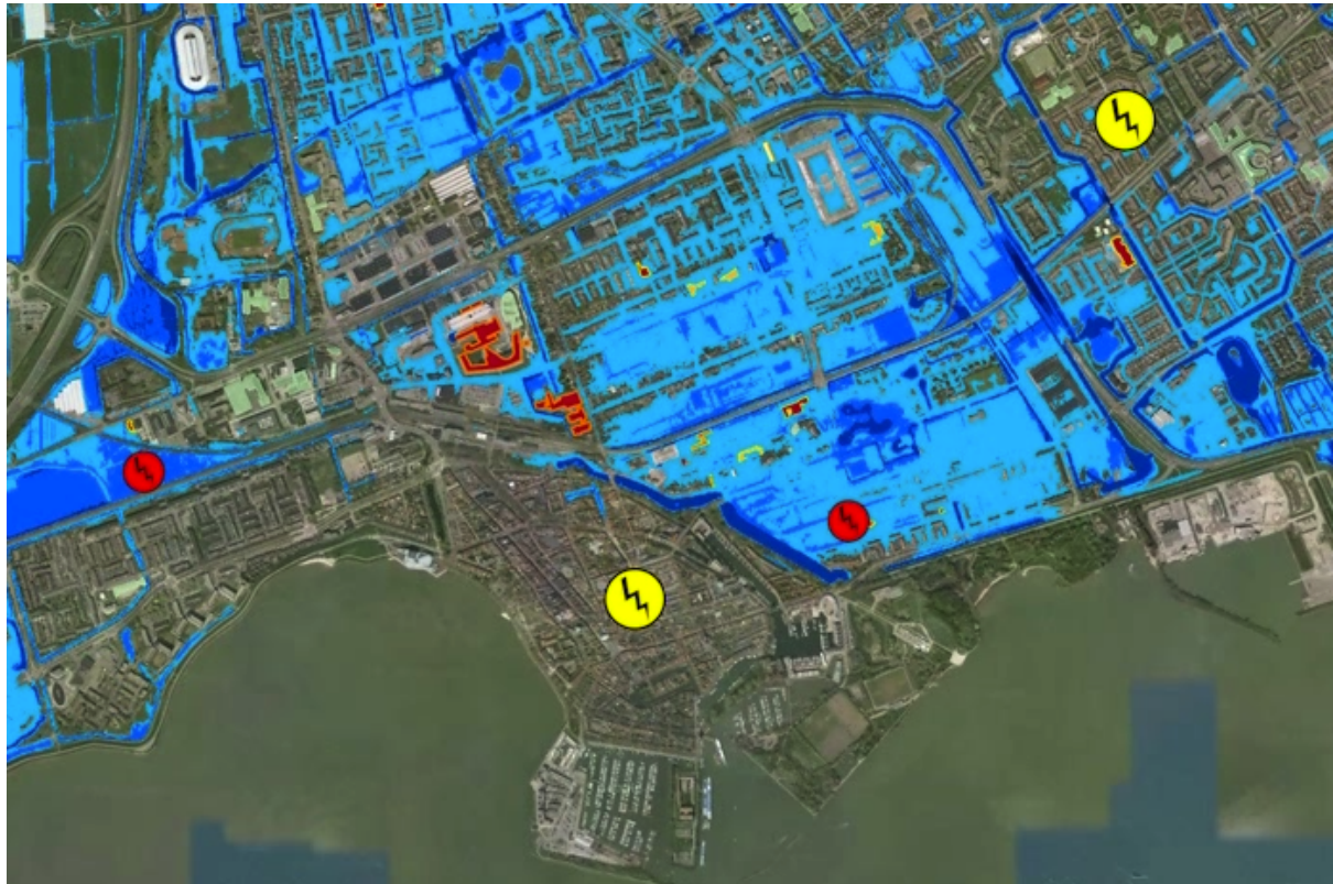
Fig. 6: Example of a layer showing electrical infrastructure impacted by flooding
