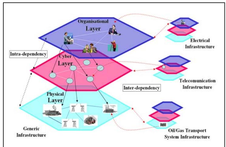
technology is to improve the dependability and survivability of large complex critical infrastructures by monitoring and protecting them with *autonomous agents* that observe mainly the working status of the *cyber-layer*, making on-line diagnostic functions, and performing recovery actions including emergency notification.
