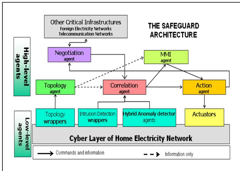
network. This is used to support the electricity state estimator to find the state of the system more reliably.
